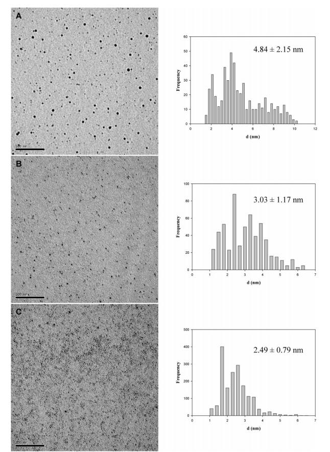
Figure 1. TEM micrographs of the AgDTC10 particles at varied initial ligand-metal feed ratios: (A) 0.5, (B) 1, and (C) 1.5. The corresponding core diameter histograms are shown to the right. The scale bars are all 100 nm.
