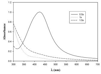
Figure 2. UV-vis absorption spectra of the three AgDTC10 nanoparticles at a concentration of ca. 1 mg/mL.
