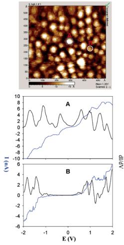
**Figure 4.** (top panel) STM topograph of AgDTC10  $(1.5\times)$  particles dispersed onto a decanethiol self-assembled monolayer that formed a priori onto a Au(111) surface. Middle and bottom panels exhibit the I-V (blue curves) and the corresponding dI/dV (black curves) profiles of two representative particles (labeled "A" and "B" in the top panel).
