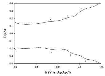
**Figure 3.** Differential pulse voltammograms of AgDTC10  $(1.5\times)$  nanoparticles at a gold electrode (area 0.1 mm<sup>2</sup>) in dichloromethane with 0.1 M tetrabutylammonium perchlorate (TBAP). Particle concentration 3.73 mg/mL. dc ramp 4 mV/s, pulse amplitude 50 mV, pulse width 200 ms. Asterisks mark the peak positions.
