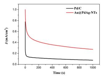
Fig. 6 Chronoamperometric curves of the Au@PdAg-NTs/GC and Pd/ C/GC electrodes in 1.0 M KOH+1 M CH<sub>3</sub>OH solution at the electrode potential of -0.15 V (vs. RHE).
