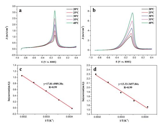
Fig. 5 LSV curves of (a) commercial Pd/C/GC and (b) Au@PdAg-NTs/GC electrodes in 1 M KOH + 1 M CH<sub>3</sub>OH solutions at different temperatures. Potential scan rate 50 mV s $^{-1}$ . Arrhenius plots of the voltammetric currents at -0.02 V (vs. RHE) with temperature for (c) commercial Pd/C and (d) Au@PdAg-NTs
