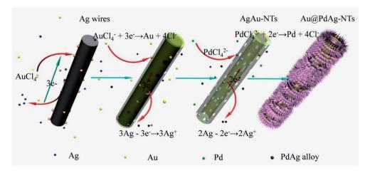
Fig. 3 Schematic illustration of the formation process of Au@PdAg-NTs by sequential galvanic replacement reactions between Ag nanowires and  $AuCl_4^-$  and  $PdCl_4^{2-}$ .
