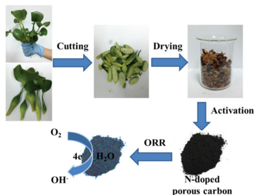
Scheme 1 Schematic of the synthesis of N self-doped porous carbon from water hyacinth.
