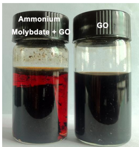
Figure S5. (left) Formation of graphene hydrogel 24 hours after the addition of ammonium molybdate at room temperature. (right) Pure graphene oxide sheets in solution without ammonium molybdate.
