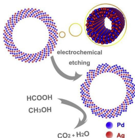
Scheme 1. Schematic illustration (cross-section view) of the as-prepared and dealloyed of PdAg catalyst of the PdAg nanotube.
