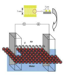
Scheme 1 Schematic of conductivity measurements of a nanoparticle monolayer at the air/water interface. Inset shows the schematic configuration of an IDA electrode. Reproduced with permission from the American Chemical Society (ref. 29).
