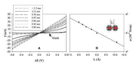
**Fig. 1** (A) I-V curves of a C4Au nanoparticle monolayer at varied edge-to-edge interparticle distances (*L*) which are shown as figure legends. The label "blank" refers to the control experiment in the absence of nanoparticle monolayers. Potential scan rate 10 mV s<sup>-1</sup>. (B) Variation of electronic conductivity with the interparticle spacings. Symbols are experimental data and line is the linear regression. Reproduced with permission from Elsevier (ref. 28).
