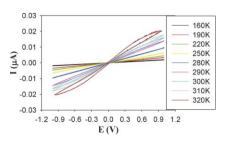
**Fig. 4** I-V profiles at varied temperatures of a C6Au monolayer deposited at L = 0.62 nm. Other experimental conditions are the same as those in Fig. 3. Reproduced with permission from Wiley (ref. 35).
