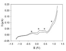
Fig. 2 I-V profile of a C6Au nanoparticle monolayer at the air/water interface with the interparticle (edge to edge) separation equal to one hexyl spacer (*i.e.*, the particles are fully intercalated). Experimental conditions are the same as in Fig. 1.
