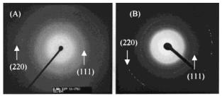
**Figure 2.** Selected area electron diffraction of the (A) as-produced and (B) thermally annealed CuC6 (rt,  $3\times$ ) particles.
