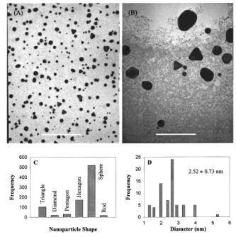
**Figure 3.** Representative TEM micrographs (A and B) of CuC6 (rt,  $3 \times$ ) particles after prolonged low-temperature thermal annealing. Scale bars (A) 100 nm and (B) 33 nm. (C) depicts the population distribution of particles of varied shapes. (D) shows the size histogram of the small particles exhibited in the background of (A) and (B).
