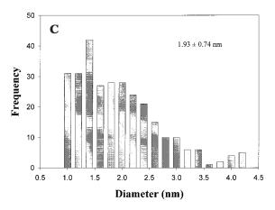
**Figure 1.** Representative TEM micrographs (A and B) of fresh CuC6  $(rt, 3\times)$  particles synthesized with superhydride as the reducing reagent. Scale bars are 51 nm. (C) depicts the particle size histogram.
