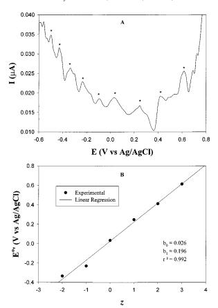
Figure 4. (A) Differential pulse voltammogram (DPV) of the asproduced CuC6 (rt, 3×) nanoparticles at a platinum disk electrode in 0.10 M TBAP in CH<sub>2</sub>Cl<sub>2</sub>. The particle concentration was ca. 3 mg/ mL. Platinum electrode area 0.01 cm<sup>2</sup>. DC ramp was 10 mV/s, pulse amplitude 50 mV. (B) Variation of formal potential  $(E_{z,z-1}^{\circ\prime})$  of the charging peaks with particle charge state (z). Symbols are experimental data and line is the linear regression.
