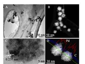
Fig. 1 Representative bright-field (A) and dark-field (B) transmission electron micrographs of Pd-CNP nanoparticles. Panel(C) depicts the high-resolution image of a Pd-CNP nanoparticle, and Panel (D) shows the elemental mapping of a pair of Pd nanoparticles where the upper curve represents the distrubition of Pd and the middle curve for C.
