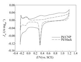
Fig. 2 Cyclic voltammograms of the Pd-CNP nanoparticles and commercial Pd black loaded onto a GC electrode in 0.1 mol·L<sup>-1</sup> H<sub>2</sub>SO<sub>4</sub> at a potential scan rate of 0.1 V·s<sup>-1</sup> (the currents were normalized by the respective mass loadings of Pd).
