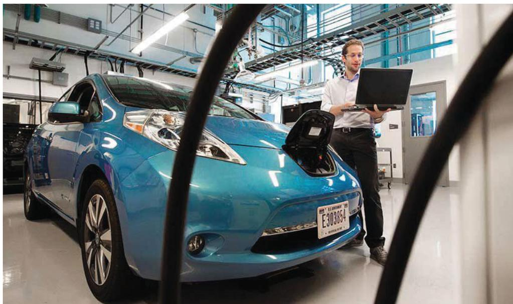
Figure 1. A new study showed that locations with clusters of plug-in electric vehicles might stress the power grid if all of the vehicles are charged at the same time. (Figure courtesy of the National Renewable Energy Laboratory.)
