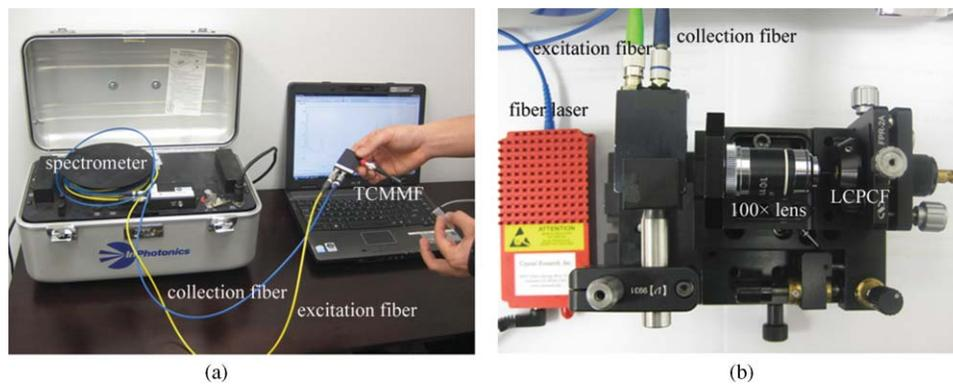
FIG. 1. (Color online) Experimental set-up: (a) TCMMF-portable SERS system; (b) LCPCF-portable SERS system (spectrometer and laptop computer not included).
