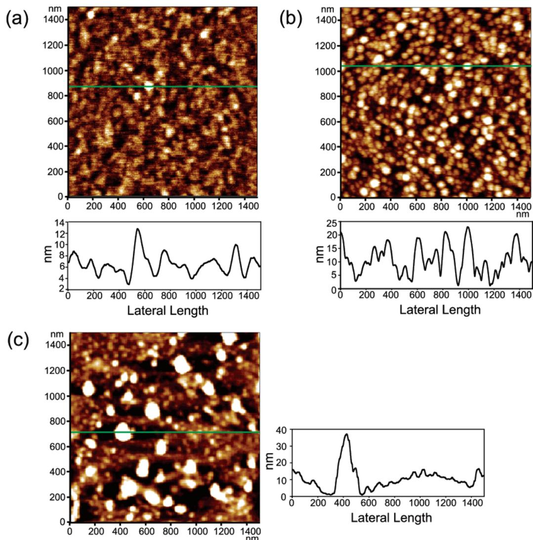
**Figure 2.** Tapping-mode AFM topographical images and representative line scan profiles of the  $\text{Fe}_{20}\text{Pt}_{80}$  nanoparticle LB films: (a) LB1, (b) LB2, (c) LB4. Scan size is  $1500 \text{ nm} \times 1500 \text{ nm}$ , and scan rate is 1.8 lines/s.
