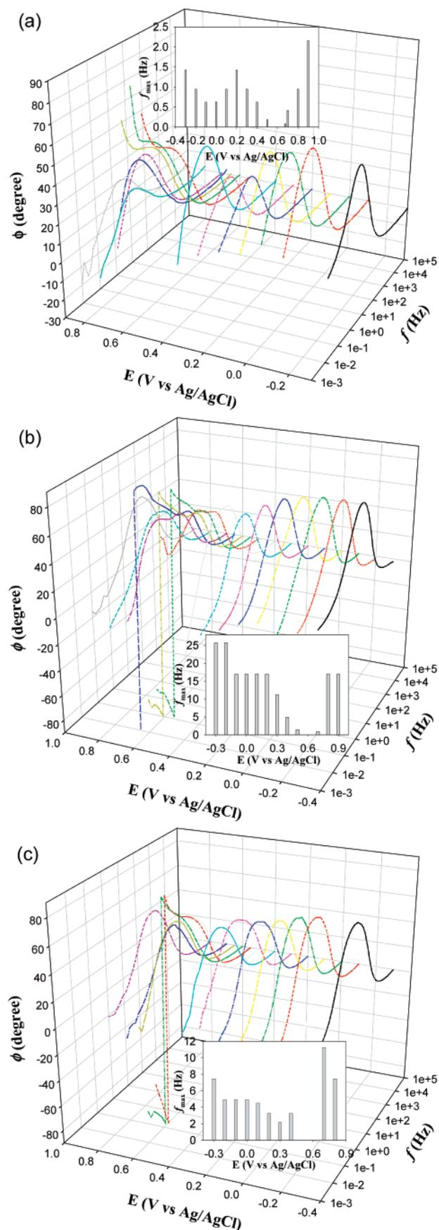
**Figure 6.** Three-dimensional Bode plots of the electrochemical impedance phase angle of the Au film electrode functionalized with different LB layers of the Fe<sub>20</sub>Pt<sub>80</sub> nanoparticles: (a) LB1, (b) LB2, and (c) LB4 in 0.1 M HCOOH + 0.1 M HClO<sub>4</sub> at various electrode potentials. Insets show the corresponding peak frequency at varied electrode potentials.
