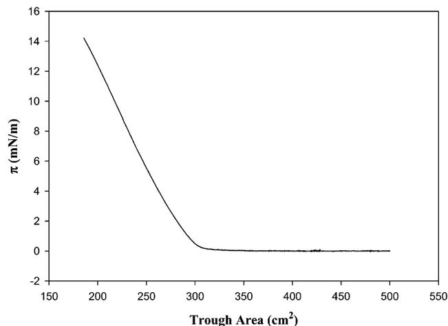
**Figure 1.** Langmuir isotherm of a Fe<sub>20</sub>Pt<sub>80</sub> particle monolayer at the air/water interface: particle concentration, 1 mg/mL in CH<sub>2</sub>Cl<sub>2</sub>; amount spread, 100  $\mu$ L; compression speed, 10 cm<sup>2</sup>/min.
