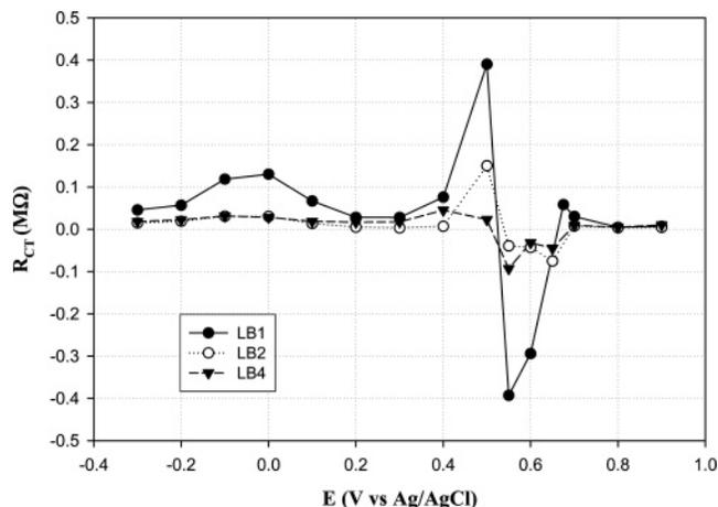
**Figure 8.** Dependence of charge-transfer resistance ( $R_{\text{CT}}$ ) on electrode potentials for the electro-oxidation of formic acid at the three particle thin film electrodes.
