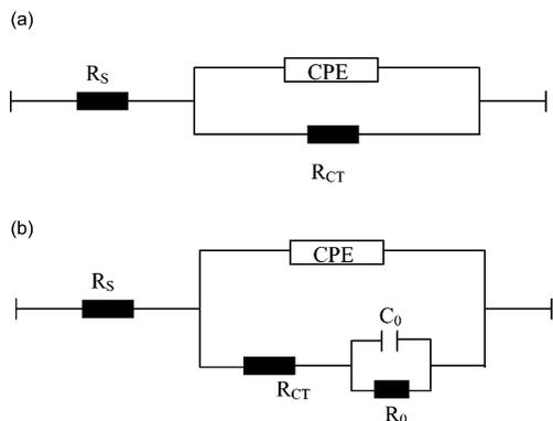
**Figure 7.** Equivalent circuits for the electro-oxidation of formic acid on the  $\text{Fe}_{20}\text{Pt}_{80}$  LB thin film electrodes: (a) for normal impedance and (b) for negative impedance shown in Figures 5 and 6.
