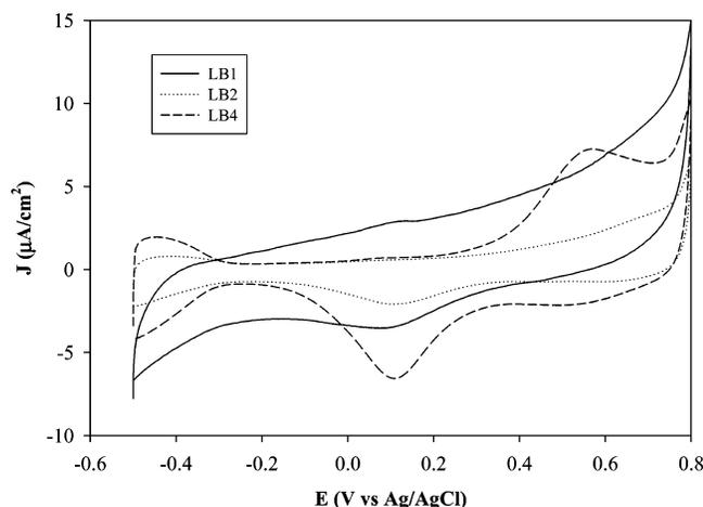
**Figure 3.** Cyclic voltammograms of the Au film electrode coated with the three different particle LB layers in 0.1 M HClO<sub>4</sub>: potential scan rate, 0.1 V/s. The currents are all normalized to the Au film surface area (0.66 cm<sup>2</sup>).
