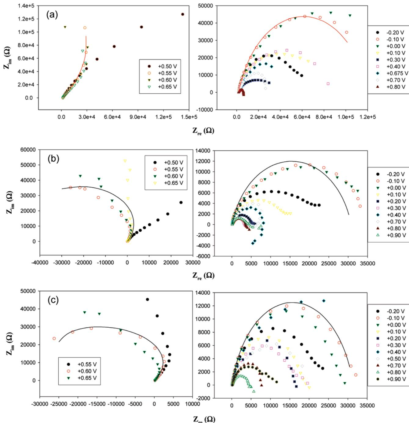
**Figure 5.** Complex-plane electrochemical impedance plots (Nyquist plots) of the Au film electrode functionalized with varied LB layers of the  $\text{Fe}_{20}\text{Pt}_{80}$  nanoparticles: (a) LB1, (b) LB2, and (c) LB4 in 0.1 M  $\text{HCOOH}$  + 0.1 M  $\text{HClO}_4$  at different electrode potentials which are shown in the figure legends. Solid lines are representative curve fits by the equivalent circuits shown in Figure 8.
