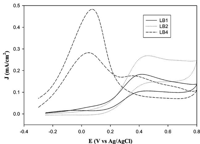
**Figure 4.** Cyclic voltammograms of the Au electrode coated with the LB1, LB2, and LB4 Fe<sub>20</sub>Pt<sub>80</sub> particle thin films in 0.1 M HCOOH + 0.1 M HClO<sub>4</sub>: potential scan rate, 0.02 V/s; gold film surface area, 0.66 cm<sup>2</sup>. The currents are all normalized to the respective Pt surface areas that are evaluated from Figure 3.
