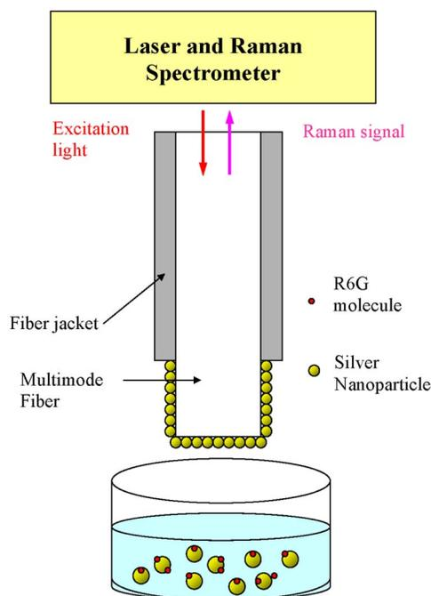
FIG. 1. (Color online) Schematic of the tip coated multimode fiber sensor.
