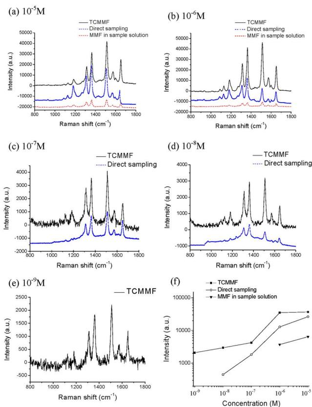
FIG. 3. (Color online) SERS spectra of R6G molecules for various concentrations by using different detection methods (TCMMF, MMF in sample solution, and direct detection). (a)  $10^{-5}M$ , (b)  $10^{-6}M$ , (c)  $10^{-7}M$ , (d)  $10^{-8}M$ , and (e)  $10^{-9}M$ . (f) Using the peak  $1514.3\text{ cm}^{-1}$  as an example, the SERS intensity vs R6G concentration is plotted.
