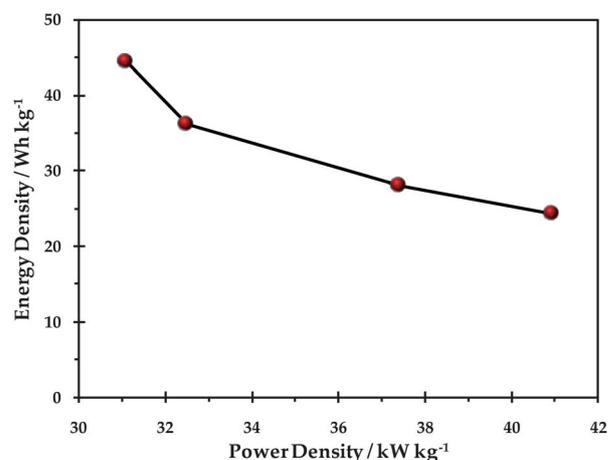
Fig. 7 Ragone plot (specific energy versus specific power density) of the GO/CoTPyzPz//GOCB based AEC.
