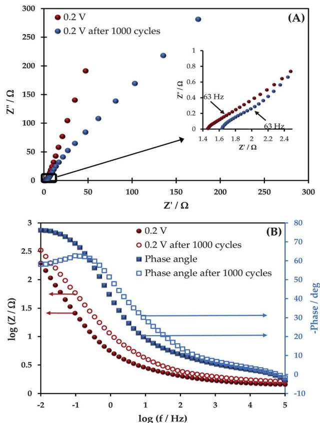
Fig. 9 (A) The Nyquist plots with an inset showing the “knee” frequencies before and after the 1000<sup>th</sup> cycle, and (B) the corresponding Bode plots of the Nyquist plots.
