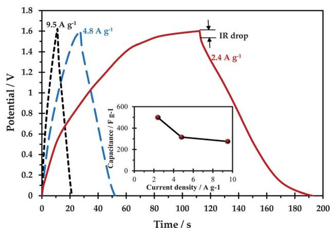
Fig. 6 Galvanostatic charge-discharge curves of GO/CoTPyzPz in 1 M Na<sub>2</sub>SO<sub>4</sub> at different current densities and the inset showing the capacitance as a function of current density.
