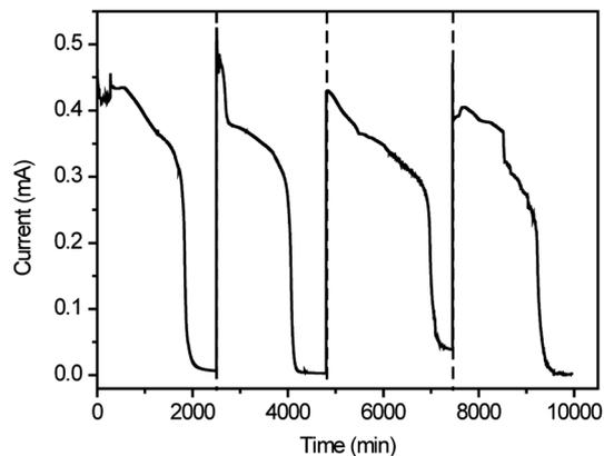
**Fig. 7** Current vs. time plot collected for a MFC device with rGO-5-Ni anode, operated in a batch-fed mode with an external resistor of 1000  $\Omega$ .
