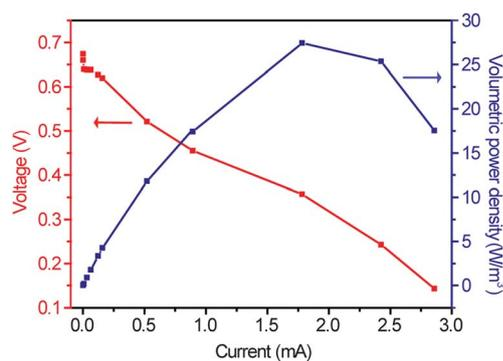
**Fig. 6** Polarization (red) and power (blue) curves collected for MFC with rGO-5-Ni anode. The volumetric power densities were calculated based on the volume of the anode chamber (~25 mL).
