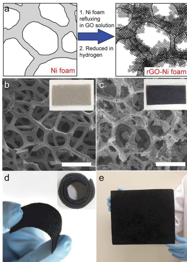
**Fig. 1** (a) A schematic diagram illustrates the preparation of rGO–Ni anode. (b and c) SEM images and digital pictures (insets) of plain nickel foam and rGO–Ni foam. Scale bars are 200 μm. (d) Digital picture of a curved rGO–Ni foam. Inset: rGO–Ni foam rolled up into a cylindrical shape. (e) Digital picture of a 25 × 20 cm rGO–Ni foam.
