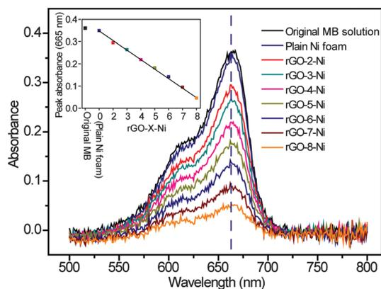
**Fig. 3** UV-vis absorption spectra collected for the original MB solution ( $2 \text{ mg L}^{-1}$  in water) and the MB solutions after reacting with rGO–X–Ni foams for 24 h. Inset: The absorption peak intensity (665 nm, highlighted by dashed line) of rGO–X–Ni foams plot as a function of the number of rGO loading cycles. A line of best-fit by eye was drawn through the data points.
