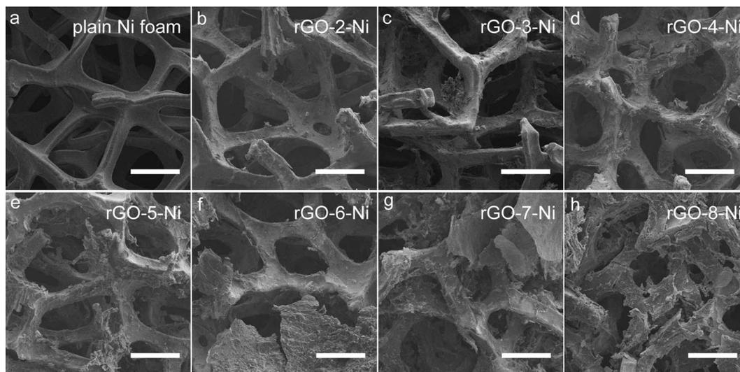
**Fig. 2** SEM images of (a) plain nickel foam, and (b–h) rGO–X–Ni (X = the number of loading cycles) foams. Scale bars are 200  $\mu\text{m}$ .
