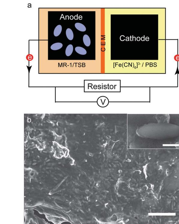
**Fig. 4** (a) Schematic diagram illustrating the configuration of a dual-chamber MFC device with MR-1 colonized bioanode and carbon cloth cathode. The anode and cathode chamber were separated by a CEM. MR-1/TSB solution was used as anolyte and ferricyanide/PBS solution was used as catholyte. (b) SEM image of an rGO–Ni anode colonized by rod-shaped *S. oneidensis* MR-1. The scale bar is 20  $\mu\text{m}$ . Inset: magnified SEM image of a MR-1 bacterium. The scale bar is 1  $\mu\text{m}$ .
