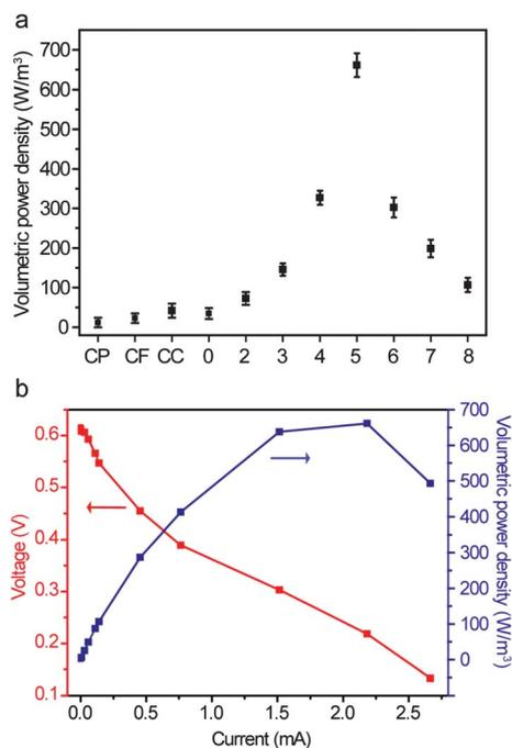
**Fig. 5** (a) Maximum volumetric power densities collected for MFC devices with rGO-*X*-Ni electrodes as anodes. Maximum volumetric power densities of MFC devices with plain nickel foam, carbon paper (CP), carbon felt (CF), and carbon cloth (CC) electrodes as anodes are also added for comparison. The error bars show the deviation of the maximum power densities for at least three devices. (b) Polarization and power curves collected for a MFC device with rGO-5-Ni anode.
